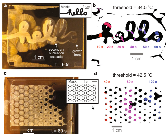
Fig. 4 Spatiotemporal evolution of thermal profiles from patterned sodium acetate trihydrate crystal growth. Temperature was monitored with an infrared camera. Precursor solution composition for all samples: 7.0 M sodium acetate, 2.8 M acrylamide, 13 mM N,N' -methylenebisacrylamide, 2 mM \alpha -ketoglutaric acid in water; 0.5 mm spacer. a Image of crystal growth in a sample that had been photopolymerized through a mask spelling out the word “hello” with light blocked within the letters. Sample was crystallized on a cold plate held at 18 °C. Full optical and thermal video available (Supplementary Movie 4). b Sum of thresholded thermal images of the sample shown in (a) . Regions that reached a threshold temperature of 34.5 °C over the course of sample crystallization are shown in black. Regions that exceeded this threshold at 10-s interval snapshots are shown in a spectrum from red to blue. c Image of crystal growth in a sample that had been photopolymerized through a hexagonal grid mask with light blocked by the lines. Sample was crystallized in air rather than on a heat sink; as such, heat was allowed to accumulate in areas where fronts converged. Full optical and thermal video available (Supplementary Movie 5). d Sum of thresholded thermal images of the sample shown in (c) . Regions that reached a threshold temperature of 42.5 °C over the course of sample crystallization are shown in black. Regions that exceeded this threshold at 40-s interval snapshots are shown in red, magenta, and blue.
