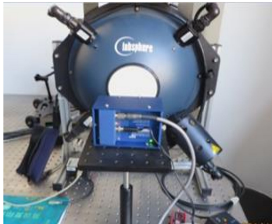
Figure 3. A photo of the uniform source system (CSTM-USS-1200C; Labsphere, Inc., North Sutton, NH, USA).
