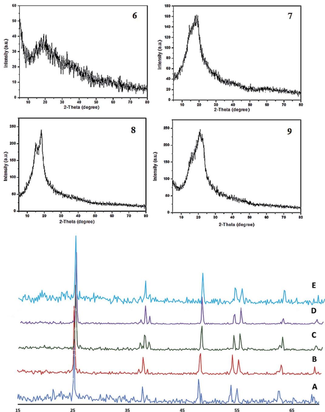
Fig. 5 X-ray diffraction patterns of heptamethine cyanine dyes **6**, **7**, **8** and **9** (top) and of Cu/TiO<sub>2</sub> (A), 9/Cu/TiO<sub>2</sub> (B), 8/Cu/TiO<sub>2</sub> (C), 7/Cu/TiO<sub>2</sub> (D), and (E) 6/Cu/TiO<sub>2</sub> (bottom).
