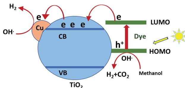
Fig. 7 Schematic of the suggested mechanism of H<sub>2</sub> production over sensitized Cu/TiO<sub>2</sub>.
