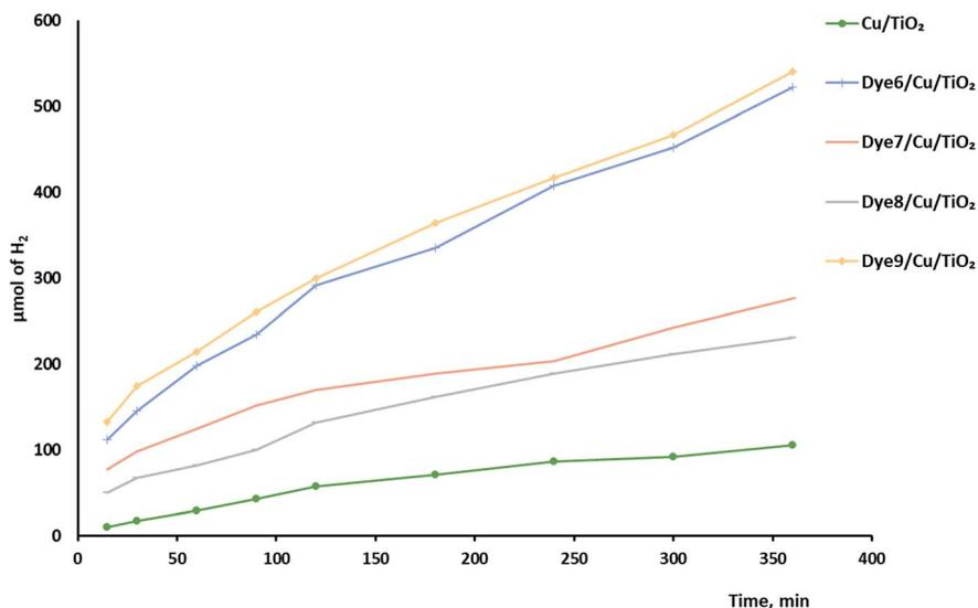
Fig. 8 Sonophotocatalytic hydrogen production over dye-sensitized Cu/TiO<sub>2</sub>.
