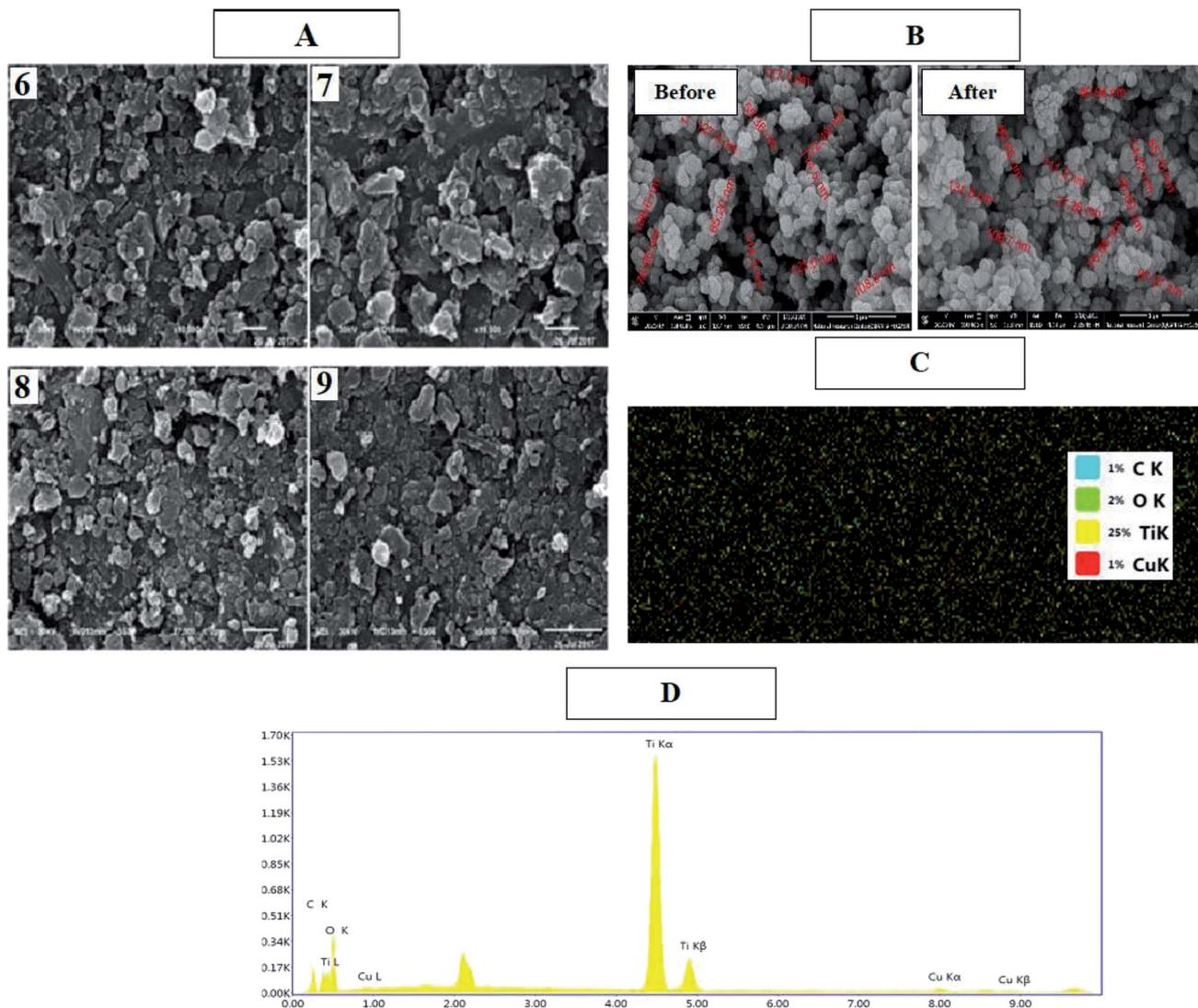
Fig. 3 SEM images of dyes 6, 7, 8, and 9 (A) and Cu/TiO<sub>2</sub> before and after sensitization (B), EDS mapping of dye sensitized Cu/TiO<sub>2</sub> (C), and EDS elemental analysis of dye 9/CuTiO<sub>2</sub> (D).
