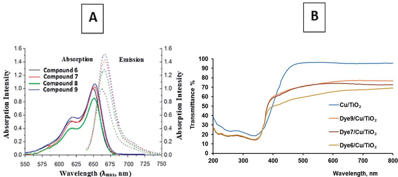
Fig. 1 (A) Absorption and emission bands of the chromophoric heptamethine carbocyanine dyes. (B) The transmittance% spectra of dye-sensitized Cu/TiO<sub>2</sub>.
