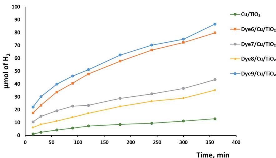
Fig. 6 The photocatalytic hydrogen production over dye-sensitized Cu/TiO<sub>2</sub>.
