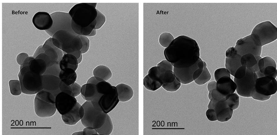
Fig. 4 TEM images of Cu/TiO<sub>2</sub> before and after dye sensitization.
