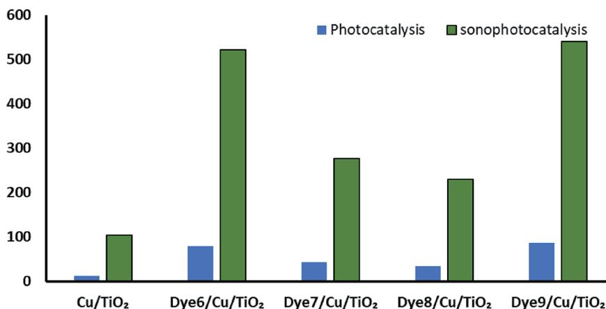
Fig. 9 Comparison between photo- and sonophotocatalytic hydrogen production.
