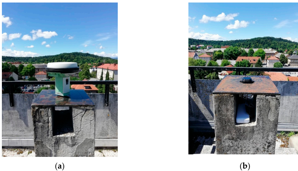
Figure 3. GNSS receivers: (a) Reference station Leica GS 15 in pillar FGG2; (b) Rover ZED-F9P in pillar FGG1.
