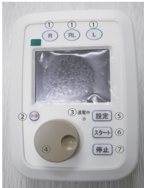
Figure 1 The portable device used for skin electrical stimulation. Each number indicates the components of the portable device. ① the button for the selection of the stimulated eye: R, right eye, RL, both eyes, L, left eye. ② The button for the emergency stop. ③ The power indicator. ④ Adjustment knob for the amount of current. ⑤ The menu button to manipulate the conditions of electrical stimulation. ⑥ The button to start electrical stimulation. ⑦ The pause button to temporarily stop electrical stimulation. If the button is hit once more, electrical stimulation will restart from the time point of the pause.
