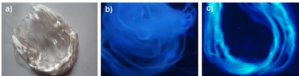
Figure 3. Optical observation of fibers: (a) fibers in visible light, (b) fibers without modifier under UV light with a 365 nm wavelength, and (c) fibers with 0.1 wt.% of KMT under UV with a 365 nm wavelength.
