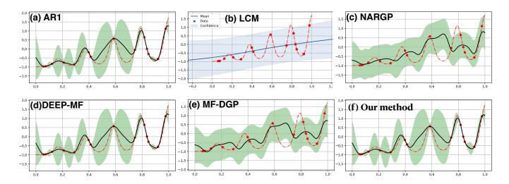
**Figure 3.** Multi-fidelity regression on the low-level true function,  $h(x) = \cos 15x$ , with 30 observations and high-level one,  $f(x) = x \exp[h(2x - 0.2)] - 1$ , with 15 observations. Top row: (a) AR1, (b) LCM, and (c) NARGP. Bottom row: (d) DEEP-MF, (e) MF-DGP, and (f) Our method with SE[SE] kernel.
