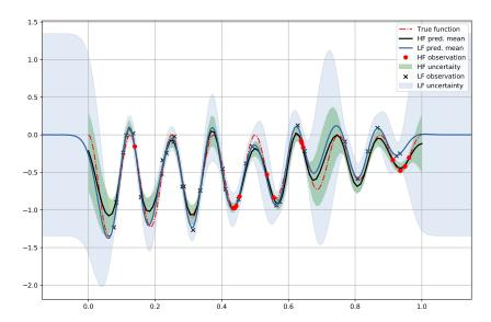
**Figure 5.** Denoising regression with 30 high-noise and 15 low-noise observations from the target function  $y = (x - \sqrt{2}) \sin^2 8\pi x$  (red dashed line). The uncertainty is reduced in the GP learning with the SE[SE] kernels.
