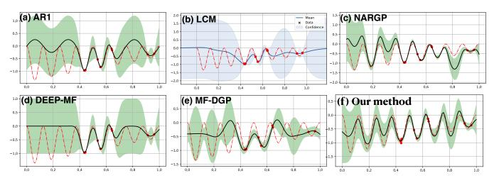
**Figure 2.** Multi-fidelity regression with 30 observations (not shown) of low fidelity  $f_1(x) = \sin 8\pi x$  and 10 observations (red dots) from the target function,  $f(x) = (x - \sqrt{2})f_1^2(x)$  (shown in red dashed line). Only the target prediction (solid dark) and associated uncertainty (shaded) are shown. Top row: (a) AR1, (b) LCM, (c) NARGP. Bottom row: (d) DEEP-MF, (e) MF-DGP, (f) our model with SE[SE] kernel.
