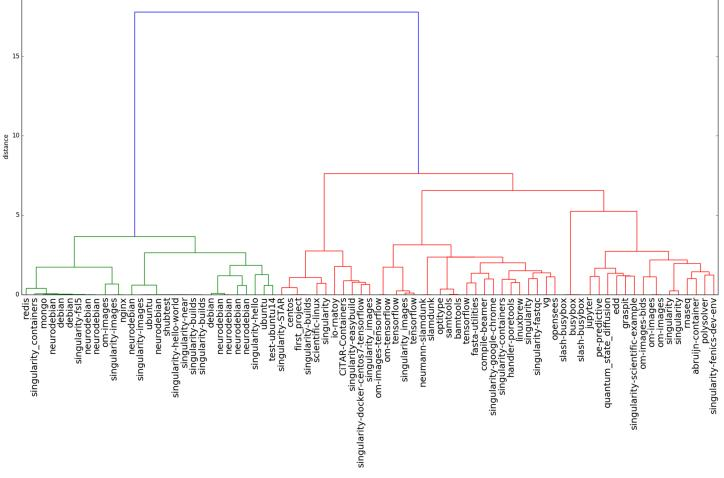
Fig 7. Hierarchical clustering of Singularity Hub public images (accessed March 28, 2017) with Ward's metric. We observed that containers generally clustered first on the level of operating systems (dark blue) in the order of Debian, Ubuntu, and then CentOS and Busybox.
