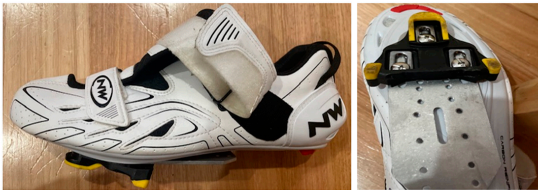
Figure 5. Northwave tri-sonic cycling shoe used in study with cleat plate securely fastened. Cleat position shown is POS with yellow Shimano SPD-SL cleat securely fastened to the cleat plate.
