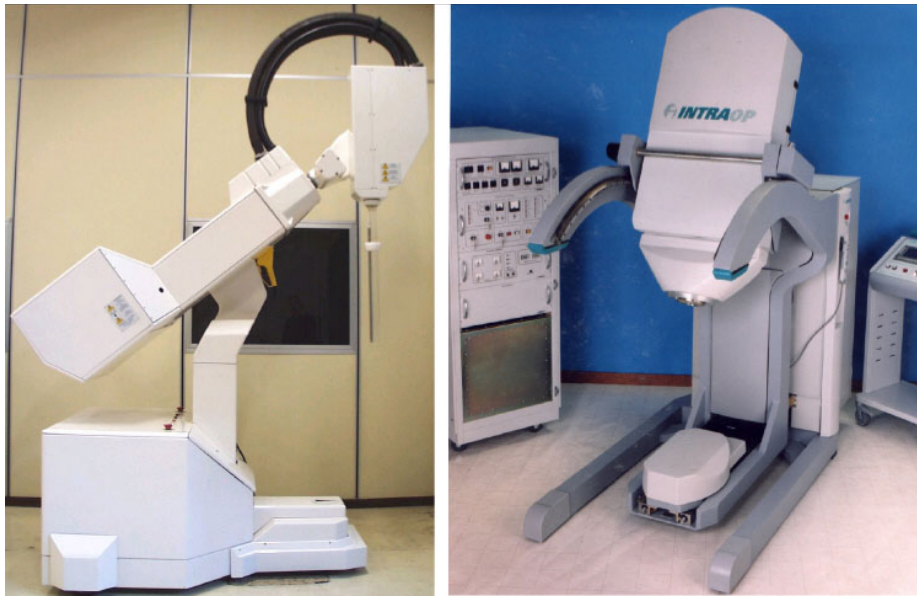
Fig. 1. The Novac7, manufactured by Hitesys (left); the Mobetron, manufactured by IntraOp Medical Incorporated (right)
