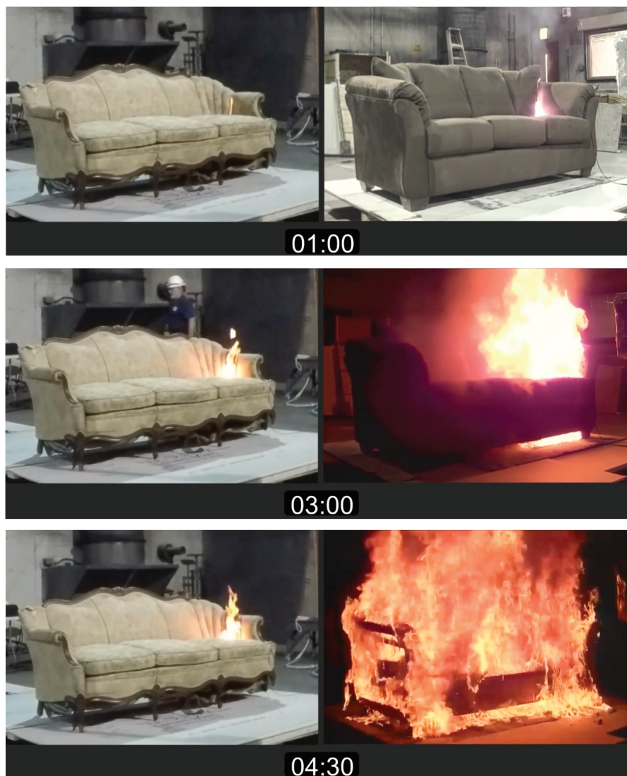
Figure 1. Set of images showing the growth rate of fires in a sofa with cotton padding (left) and in a sofa with polyurethane foam and polyester padding (right). Three times are shown after ignition of the fire starting from the top: 1, 3, and 4.5 minutes.
