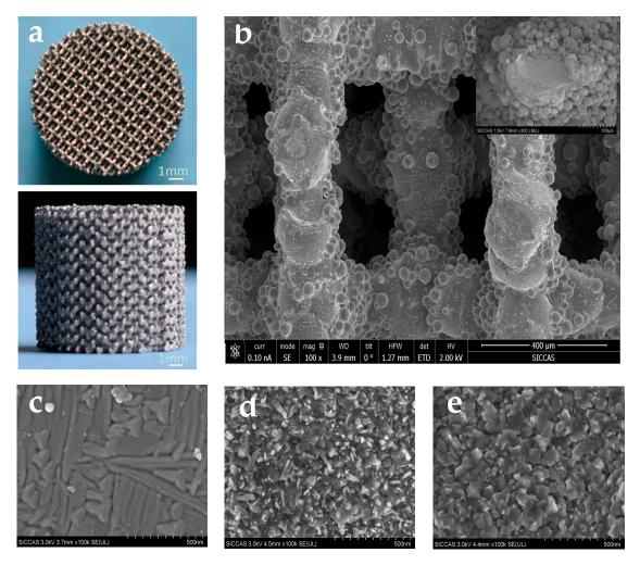
**Figure 1.** Overview of Ti-6Al-4V scaffolds (a); low-magnification view of scaffold struts showing macro pore sizes around 0.5 mm (b) together with an inserted high-magnification SEM image of the surface morphology of Ti-6Al-4V scaffold struts (c); BG-coated Ti-6Al-4V scaffold struts (d) and MBG-coated Ti-6Al-4V scaffold struts (e).
