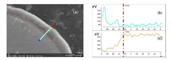
Figure 2. Cross-section morphology (a) of MBG-coated Ti-6Al-4V scaffold strut showing an interlayer and the MBG coating layer with a thickness of about 1  $\mu m$  and EDS line scan analysis (from the red dot to the blue dot) showing interdiffusion of Si (b) and Ti (c) across the interlayer between the coating layer and substrate.
