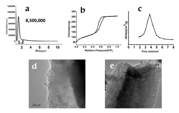
**Figure 3.** Grazing incidence X-ray diffraction (GIXRD) pattern of the MBG-coated Ti-6Al-4V scaffolds (a); nitrogen adsorption—desorption isotherms of the MBG powder (b); pore size distribution extracted from the N2 adsorption isotherms of the MBG powder (c); and TEM images for the MBG-coated Ti-6Al-4V scaffolds (d,e) with a well-ordered mesopore channel structure.
