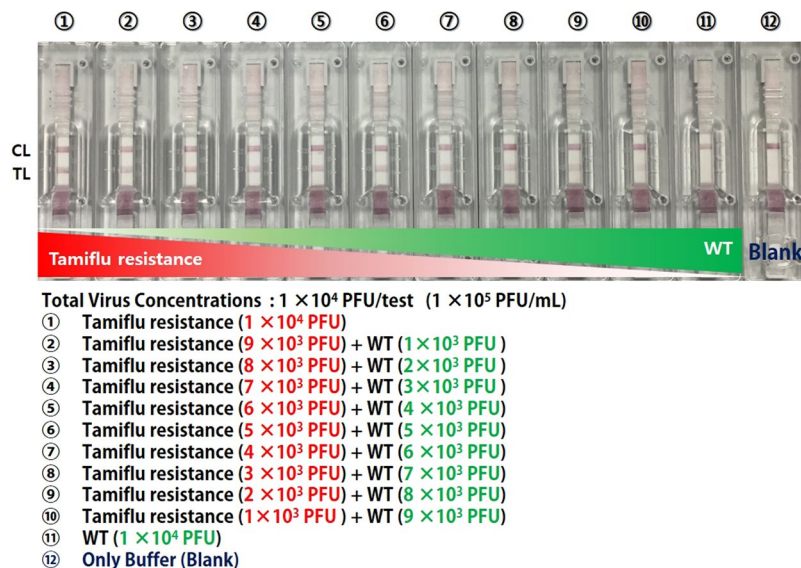
Figure 8. Specificity analysis of Tamiflu resistance detection using an OHT-based lateral flow assay (LFA) at various ratios of WT and Tamiflu-resistant viruses within 10 min. Mixed buffer containing Tamiflu-resistant and WT viruses is dropped onto a loading zone (sample pad) of the LFA. After 10 min, the test line (TL) appears darker as the concentration of the Tamiflu-resistant virus increases. Blank (buffer only) is used as a control. The control line (CL) indicates that this OHT-based LFA is operating correctly.
