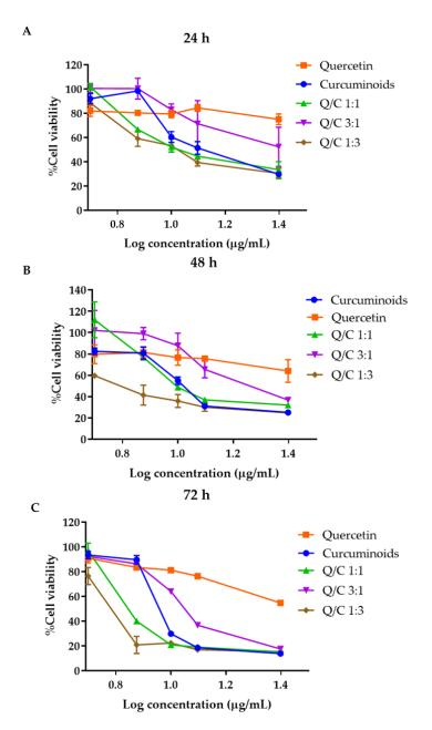
**Figure 3.** HDFB cell viability after treatment with quercetin, curcuminoids and quercetin/curcuminoid mixtures and further incubated for (**A**) 24 h, (**B**) 48 h and (**C**) 72 h.
