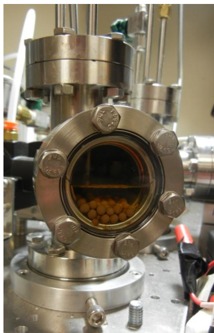
Figure A5. Solvent reservoir with optical view port, liquid solvent, and molecular sieves.
