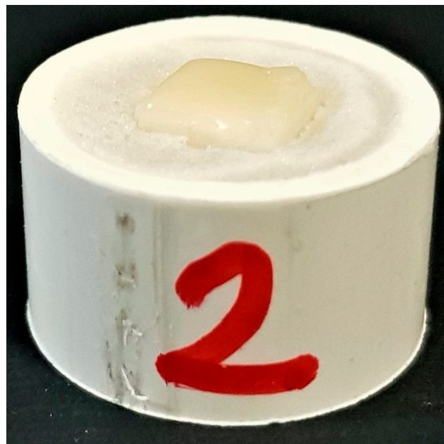
Figure 1. Zirconia specimen layered with ceramic and embedded in a resin block.
