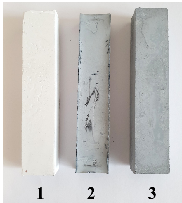
Figure 2. Photograph of prepared prismatic specimens of (1) MOC-REF (a reference sample with pure Magnesium Oxychloride Cement), (2) MOC-G (Magnesium Oxychloride Cement with Graphene), and (3) MOC-G-H (Magnesium Oxychloride Cement with Graphene Homogenized by Ultra-Turrax).
