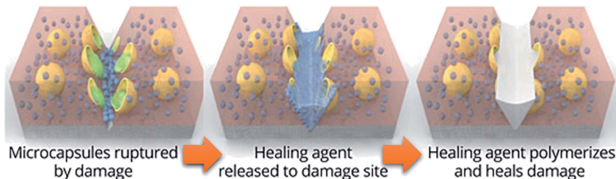
Fig. 2 Concept of self-healing based on microencapsulated healing agent (in yellow) embedded in a matrix (in red) containing a catalyst (in blue) capable of polymerizing the healing agent (in green). 10,11
