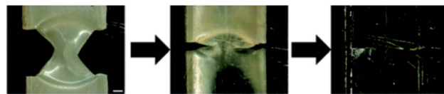
Fig. 15 Shape memory assisted self-healing of macroscopic damaged using thermally healable crosslinked/linear PCL fibers. 131,132
