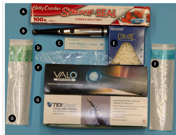
Fig. 1. Materials used in this study: six different infection control barriers and one multi-peak LCU. A- Stretch and Seal Flexible Film (Betty Crocker); B- VALO Grand light curing unit (Ultradent); C- Cure Sleeve by Pinnacle (Kerr); D- Disposa-Shield (Dentsply Sirona); E- Curelastic (Steri-Shield); F- VALO Grand Disposable Barrier Sleeves (Ultradent); G- TIDIShield Curing Light Sleeves (TIDI Products).
