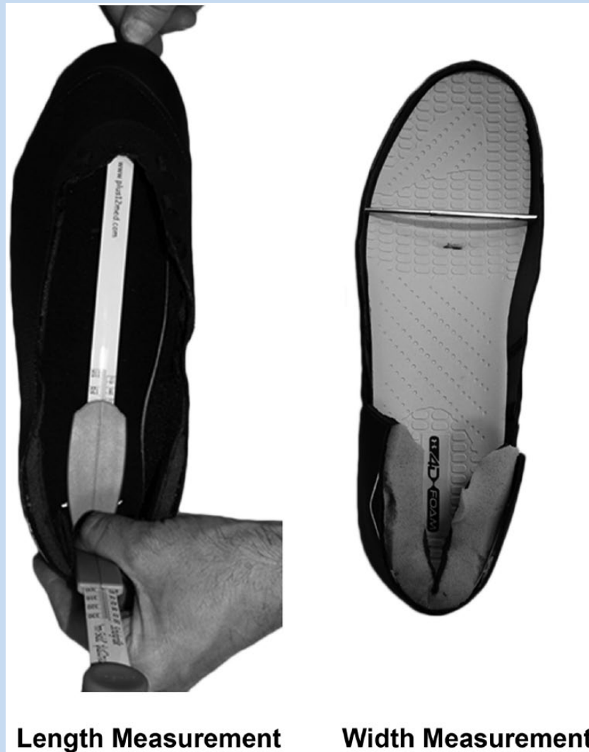
Figure 2. Photographs of shoe length measurement using the PlusMed12 device (left) and width measurement using the telescoping rod at 70% of the footwear length from the heel (right).
