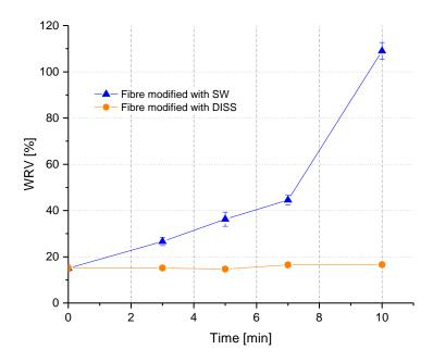
Figure 10. Water retention value vs time of treatment using DISS and SW.
