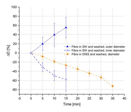
Figure 9. Changes in fibre diameter over time after washing.
