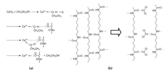
**Figure 1.** Proposed complexation mechanism of polyamide 6.6 (PA 6.6) in CaCl<sub>2</sub>/EtOH/H<sub>2</sub>O solvent: (a) Complex formation; (b) Disruption of hydrogen bonds in PA 6.6 in the presence of CaCl<sub>2</sub> according to [24].
