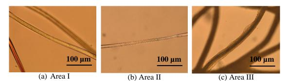
**Figure 2.** Pictures of the PA 6.6 fibres treated with solvents of the corresponding area: (**a**) No effect of the solvent on the fibres; (**b**) Dissolution of the fibre surface leading to fibre thinning (DISS); (**c**) Formation of a swollen shell (SW).
