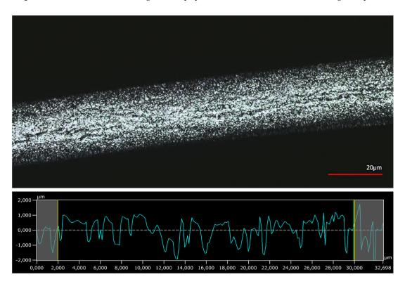
**Figure 13.** 3D confocal laser-scanning microscope picture of PA 6.6 fibre modified using SW and roughness profile.
