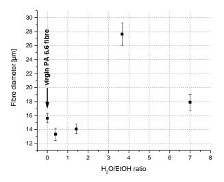
**Figure 7.** Fibre diameter as a function of  $H_2O/EtOH$  ratios in CaCl<sub>2</sub>/ $H_2O/EtOH$  mixtures after 10 min treatment.
