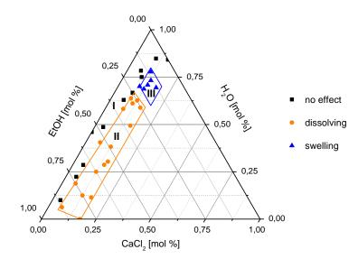
Figure 3. Ternary phase diagram of the CaCl<sub>2</sub>/H<sub>2</sub>O/EtOH system for PA 6.6 fibre treatment.
