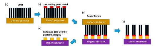
**Figure 2.** Schematic of CNT transfer method: (a) vertically-aligned CNT growth; (b) evaporation of low-melting point metal such as solder through hard mask onto CNT array; (c) preparation of target substrate; (d) solder reflow process to bond the CNT array and target substrate; (e) separation of CNT array from donor substrate.
