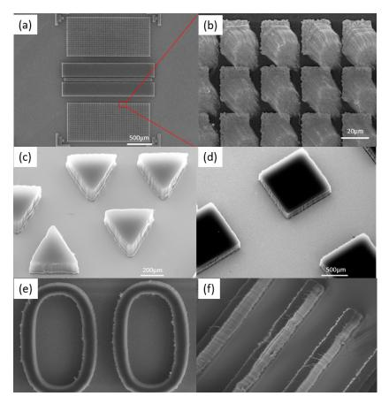
**Figure 3.** (a,b) Transferred CNT with bump size of 25  $\mu$ m and a pitch of 10  $\mu$ m with surrounding bumps; (c-f) multiple shapes of transferred CNT—for (e,f) the width of the CNTs patterns are 200  $\mu$ m and the height of the CNT 500  $\mu$ m.
