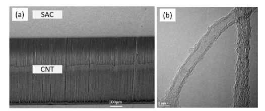
**Figure 1.** (a) Silver-copper alloy (SAC) deposited on vertically-aligned carbon nanotube (VACNT) does not affect the alignment of the array; (b) Transmission electron microscopy (TEM) image of as-grown CNT.
