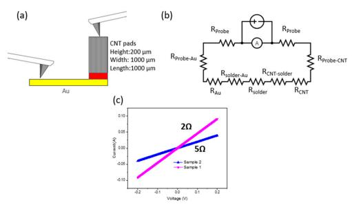
**Figure 4.** (a) Measurement setup to measure IV-response of transferred CNT array at given CNT dimension; (b) schematic of electrical connection in measurement setup; (c) measured IV-responses and corresponding resistances.
