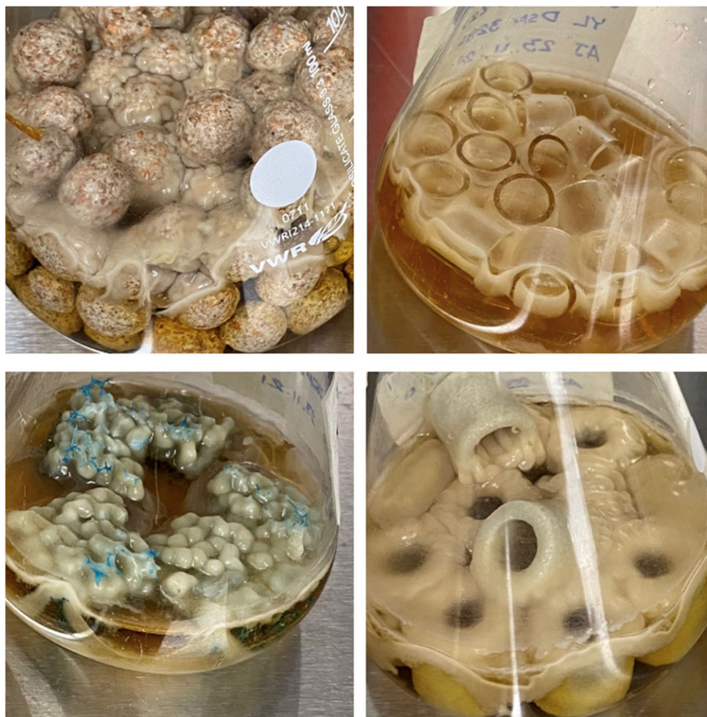
Figure 2. Biofilm formation of Y. lipolytica strain DSM3286 on the liquid/gas interface using YPG medium while applying different solid materials as a support, including (A) ceramic, (B) glass tube, (C) nylon, and (D) sintered glass.
