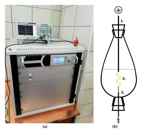
**Figure 7.** Set-up of generator and reactor for HVED treatments: (a) HVED and plasma generator "IMP-SSPG-1200" (Impel group d.o.o., Zagreb, Croatia); (b) Beaker shaped reactor: (1)—ground electrode; (2)—high voltage electrode (needle with empty interior for argon and nitrogen flow) during treatments; and (3)—discharge (plasma).
