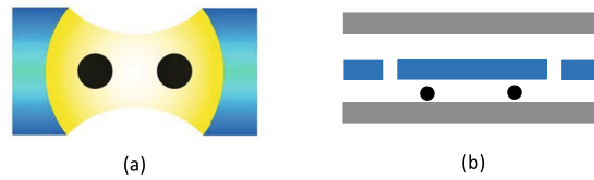
Figure 1. (a) Setup for two superconducting transmon qubits embedded in a 3D cavity. (b) Setup for two superconducting transmon qubits coupled to a 1D transmission line resonator. A dark dot represents a superconducting transmon qubit.
