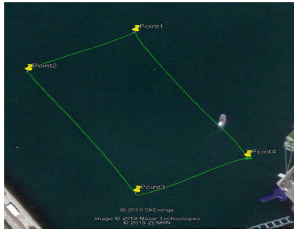
Figure 23. Waypoint tracking control results.
