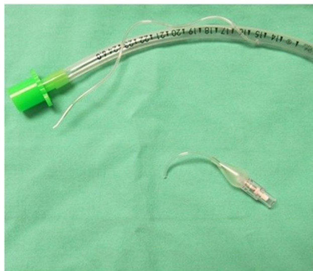
Figure 1 Severed pilot balloon, separated from the tubing of a cuffed endotracheal tube.
