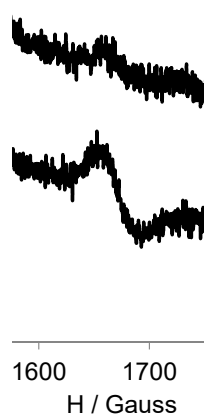
Figure 4. EPR spectra of |\Delta m_s| = 2 transition at half-field for the same concentration 10^{-4} M of G0-OEG-PROXYL and G1-OEG-PROXYL at 120 K in \text{CH}_2\text{Cl}_2 .
