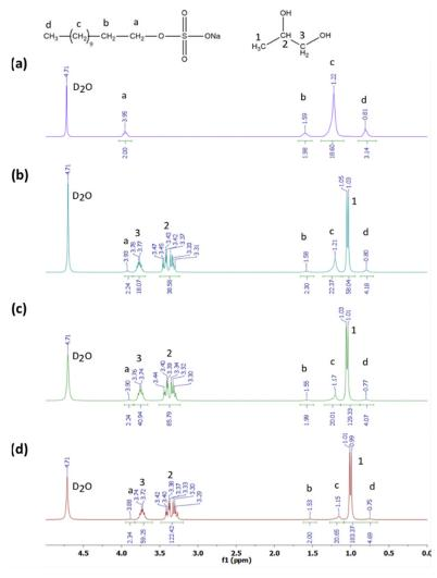
**Figure 3.**  $^{1}$ H NMR results of SDS (0.01 mol dm $^{-3}$  SDS solution) in the binary mixture of water and (a) 0 mass fraction of propane-1,2-diol, (b) 0.05 mass fraction of propane-1,2-diol, (c) 0.10 mass fraction of propane-1,2-diol and (d) 0.15 mass fraction of propane-1,2-diol.
