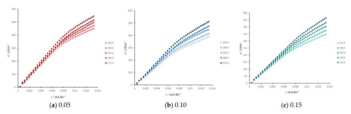
**Figure 1.** Plot of electrical conductivity vs. concentration for SDS in the binary mixture of water–propane-1,2-diol at different temperatures, where the mass fraction of propane-1,2-diol is equal to (a) 0.05, (b) 0.10 and (c) 0.15.
