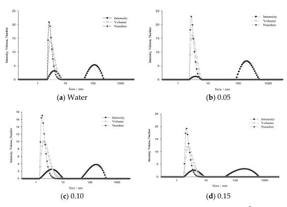
**Figure 2.** Dynamic light scattering (DLS) measurement of the size distribution of SDS (0.01 mol dm $^{-3}$  SDS solution) in the binary mixture of water and (a) 0 mass fraction of propane-1,2-diol, (b) 0.05 mass fraction of propane-1,2-diol, (c) 0.10 mass fraction of propane-1,2-diol and (d) 0.15 mass fraction of propane-1,2-diol.
