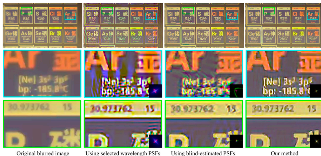
Figure 9. Results for the periodic table image. The top-left image is the captured blurred image. The right three images on the top row are the restored results using three sets of spatially varying PSFs. The bottom two rows are the details of the top-row images. The bottom-right corners of the detail images of the restored results show the used local PSFs.
