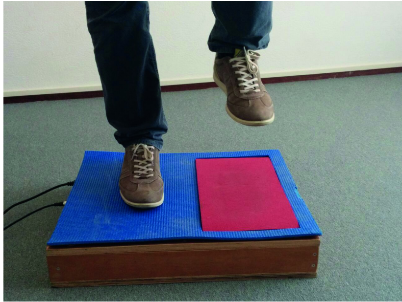
Fig 1. Stamping on the force-sensitive area of the force plate.
