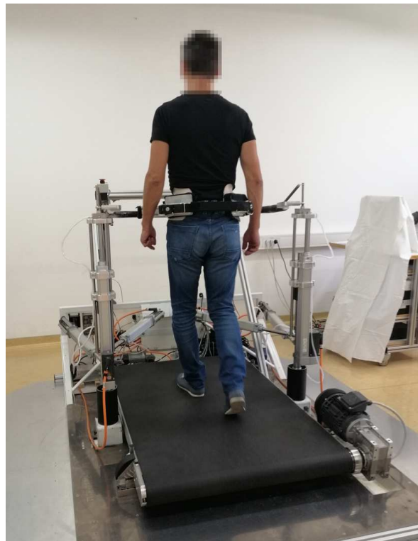
Figure 1. A healthy individual walking on an instrumented treadmill while being embraced by the Balance Assessment Robot for Treadmill walking - BART, which enables perturbations to the subject's pelvis.
