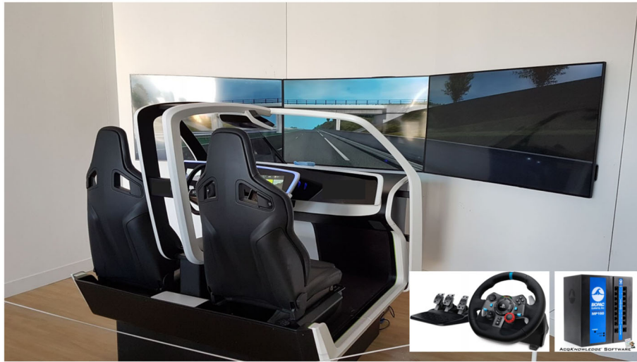
FIGURE 3 Overview of the equipment: homemade driving simulator, Biopac MP160 data acquisition system, Logitech G29 steering wheel and pedals
