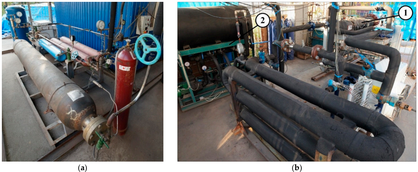
Figure 2. Experimental setup for study of natural gas charging and discharging processes from ANG storage system: (a) high pressure gas preparation unit and (b) circulating charging unit including adsorption tank (1) and coolant preparation unit (2).
