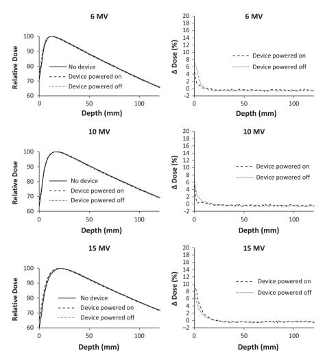
**Fig. 4.** %DD of 10 cm  $\times$  10 cm photon beams of nominal energy 6 MV (top), 10 MV (middle), and 15 MV (bottom). %DDs were measured with and without the quality monitoring system in place and with it powered on and powered off.  $\Delta$  Dose (%) represents the percent difference from the %DD of the beam without the device in place.
