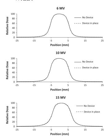
**Fig. 7.** Inline beam profiles at 10 cm depth for  $1\times 1$  cm<sup>2</sup> photon beams of nominal energy 6 MV (top), 10 MV (middle), and 15 MV (bottom). Profiles were measured with and without the quality monitoring system in place.
