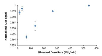
**Fig. 3.** Normalized IQM signal measured from a 50 MU  $10~\text{cm} \times 10~\text{cm}$  6 MV photon beam delivered at various dose rates. The measurements are normalized to the highest dose-rate measurement with a Farmer chamber used as a reference measurement.
