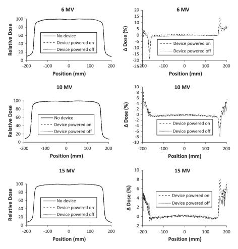
**Fig. 5.** Beam profiles at 10 cm depth on the MLC motion axis of 30 cm  $\times$  30 cm photon beams of nominal energy 6 MV (top), 10 MV (middle), and 15 MV (bottom). Profiles were measured with and without the quality monitoring system in place and with it powered on and powered off.  $\Delta$  Dose (%) represents the percent difference from the profile of the beam without the device in place.
