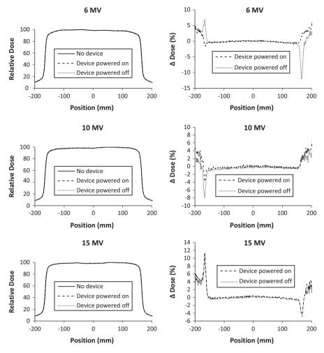
Fig. 6. Beam profiles at 10 cm depth perpendicular to the MLC motion axis of 30 cm  $\times$  30 cm photon beams of nominal energy 6 MV (top), 10 MV (middle), and 15 MV (bottom). Profiles were measured with and without the quality monitoring system in place and with it powered on and powered off.  $\Delta$  Dose (%) represents the percent difference from the profile of the beam without the device in place.
