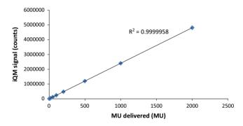
Fig. 2. IQM signal shows linear dependence on the MU delivered for a 6 MV 10 cm  $\times$  10 cm photon beam.
