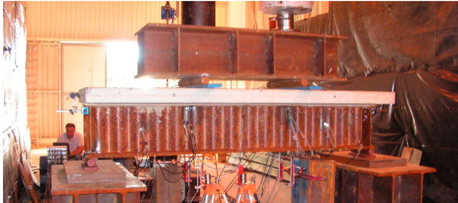
Figure 3. View of the typical four-point bending test setup.
