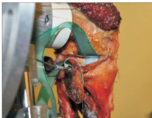
Fig. 2. Photograph of a Tekscan pad inserted posteriorly in the medial tibiofemoral joint space.
