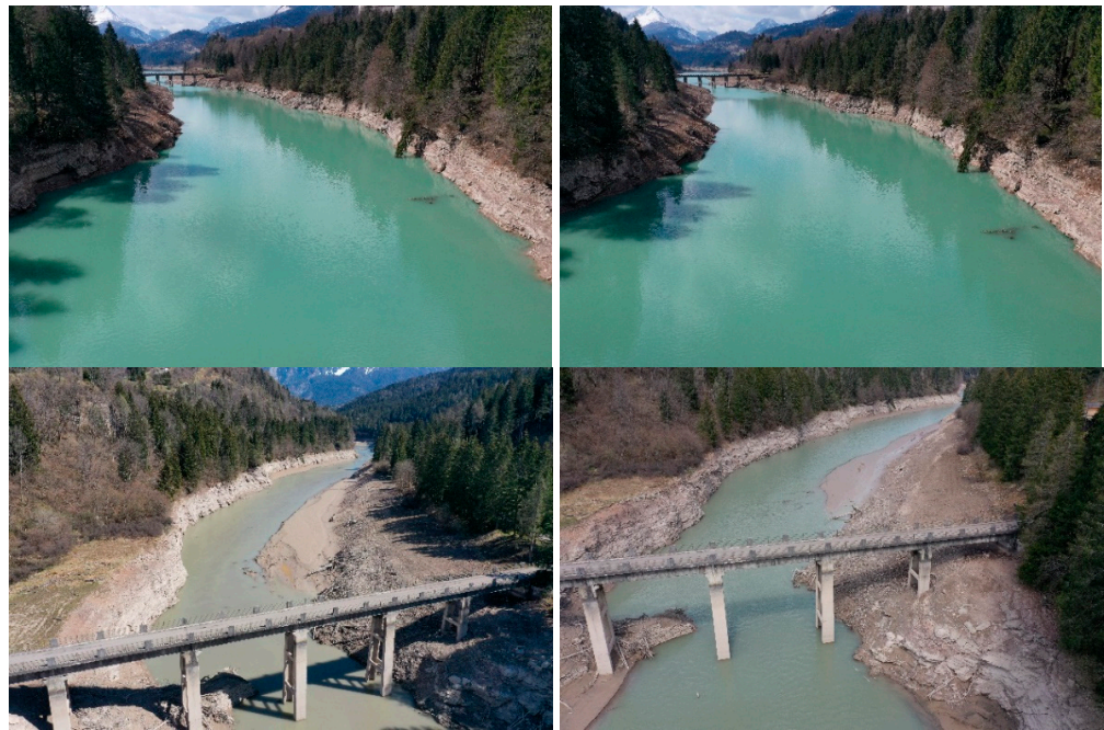
Figure 3. Example of images recorded by the UAV with FOV = 77° and gimbal pitch angle = 45°.
