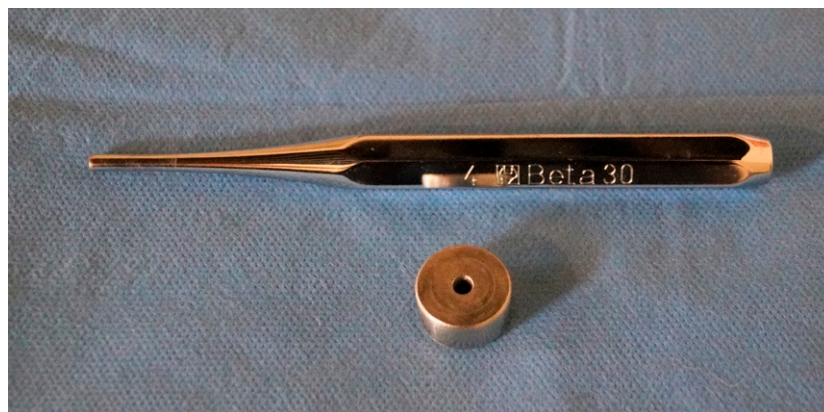
Figure 1. Reusable cylindrical stainless-steel mold with an orifice of 4 mm in diameter and 10 mm in depth. The hole was entirely filled with each of the studied materials, taking care of fully fill the internal space and avoiding the creation of possible voids.
