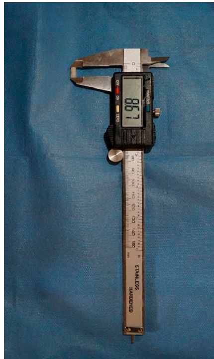
Figure 3. Digital caliber of \pm 0.1 mm accuracy (Qfun) used to measure the absolute length of the specimen of cured composite.
