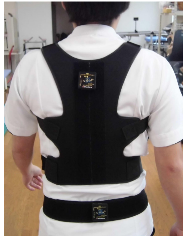
Fig. 1 Two-point gait oscillometer MVP-WS2-S. Two compact wireless sensors were attached to the dorsal vertebral region and the sacral region with the specified harness and belt
