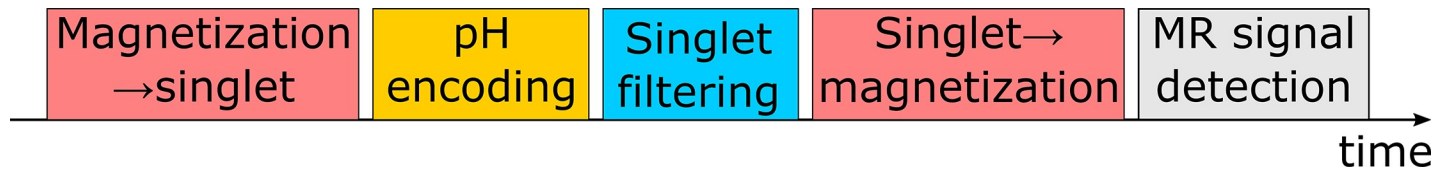
Fig 1. Suggested 5-step SISTEM pulse sequence: (1) magnetization of ^1\text{H} nuclei is transferred to LLs and zero-quantum coherences; (2) encoding a feature (here: Chemical shift difference that can be correlated with the pH value, Figs 4 and 5); (3) background suppression: Only singlet spin states (or zero-quantum coherences) pass through the filter; (4) conversion of singlet state into observable magnetization and (5), MR signal detection.
