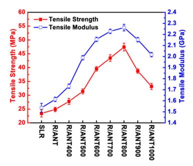
**Figure 6.** The complete dataset of tensile strength and elastic modulus of stereolithography (SLA) 3D printed samples prepared with the fillers of annealed anatase TNPs at different heat-treated temperatures.
