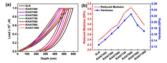
**Figure 8.** (a) Indentation load-depth curves for 3D printed samples of neat SLR and SLR/nanofillers composites. (b) The reduced modulus and hardness of 3D printed samples of SLR and SLR/nanofillers composites.
