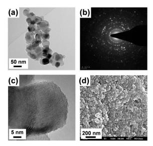
**Figure 5.** (a,c) High-resolution transmission electron microscopy (HRTEM) image of ANT800 NPs. (b) Selected area diffraction pattern (SAED) of ANT800 NPs. (d) Field emission scanning electron microscope (FESEM) image of ANT800 NPs.
