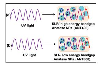
**Figure 2.** The key mechanism of photopolymerization process assisted by UV light penetration through the (a) stereolithography resin (SLR)/high energy bandgap semiconducting anatase nanoparticles (NPs) (ANT400) and (b) SLR/low energy bandgap semiconducting anatase NPs (ANT800). The energy/intensity of UV rays reduced (the violet color lines indicate higher intensity and red color lines indicates lower intensity) when it underwent deep penetration through the resin composites.
