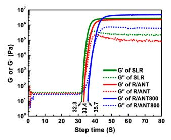
**Figure 10.** The effects of nanofillers on the kinetics of UV curing reaction. The solid and dotted lines represent storage modulus (G') and loss modulus (G'') of the samples during the curing process, respectively.
