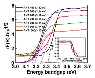
**Figure 14.** Tauc's plot for an indirect bandgap model (Kubelka-Munk function) and UV-visible diffusive reflectance spectra (inset) of annealed anatase TNPs. The dash-dot lines represent line tangent towards the point, where the line intersected the horizontal energy axis (bandgap). The observed bandgap of controllably annealed anatase TNPs is mentioned in brackets, followed by the sample name.
