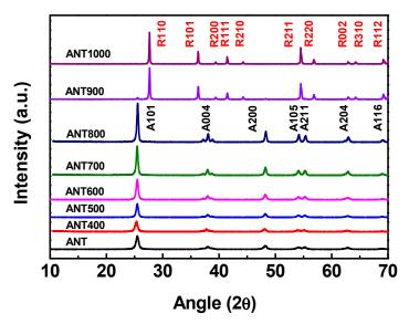
**Figure 3.** X-ray diffraction peaks of anatase TNPs annealed at different temperatures. The R and A represent the rutile and anatase phase, respectively, where the number followed by the R or A represents the crystal plane.
