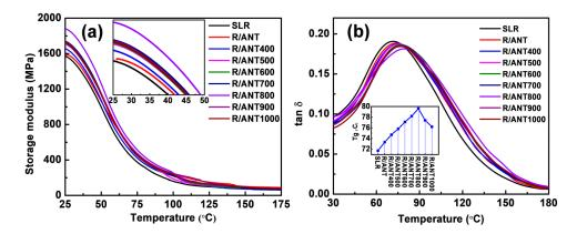
**Figure 9.** Thermo-mechanical analyses of neat SLR and SLR/nanofillers 3D printed samples. (**a**) Storage modulus and (**b**) tan  $\delta$  curves. The inset in (**a**) shows the enlarged view of dynamic mechanical analysis (DMA) curves at a horizontal axis between 25 °C and 50 °C, and the inset in (**b**) shows the observed glass transition temperature ( $T_g$ ) of different samples from the tan  $\delta$  curve.
