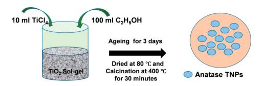
Figure 1. A detailed schematic route of anataseTiO<sub>2</sub> nanoparticle (TNP) preparation by sol-gel method.
