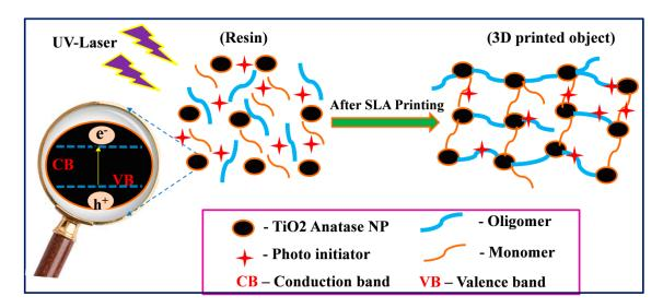
**Figure 15.** A schematic illustration of photopolymerization of photo resin with semiconducting anatase TNPs under UV light for the SLA 3D printing.
