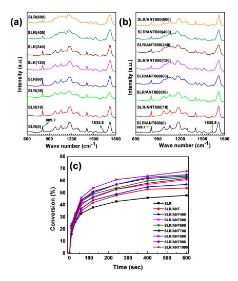
**Figure 13.** A real time FTIR analysis of photopolymerization of neat SLR and SLR/ANT800. (a) Neat SLR and (b) SLR/ANT800 nanofillers composite in different periods of UV irradiation time intervals starting from 0 s to 600 s. (c) Percent conversion graph of neat SLR and SLR/nanofillers.
