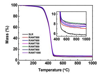
**Figure 11.** The thermal stability analysis for 3D printed samples of neat SLR and SLR/nanofillers 3D printed samples. The inset shows the enlarged view of the curves between 400 °C and 1000 °C to understand the final residual char values.
