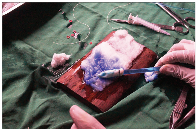
Figure 6: Measurement of bursting pressure. The pressure was recorded when the bond broke characterized by blue stream of solution escaping and sudden drop in pressure
