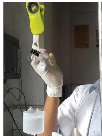
Figure 4: Measurement of breaking load. It was measured when the bond gave way and a gap was seen
