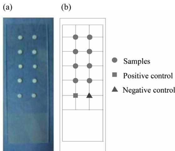
**Fig. 6.** The arrayed aerogel dots on a glass slide. Left: the real object. Right: the corresponding experimental design layout. The positive and negative control spots validated the experimental process. Cy3–Sp5 served as the positive control and the immobilization buffer served as the negative control.
