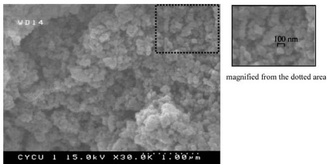
**Fig. 5.** SEM image of the silica aerogel. The image shows that the surface is formed by a great number of silica nanoparticles with an average size of around 100 nm. The rough surface and interstitial space among particles provided a vast amount of capturing sites available for biological samples. The image was magnified in 30 k-folds.
