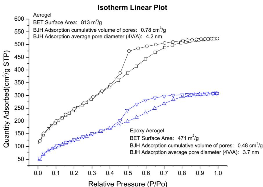
**Fig. 4.** Nitrogen isotherm of the silica aerogel product. The isotherm exhibited a type-IV curve and the measurement indicated that its specific surface area was  $813\text{ m}^2\text{ g}^{-1}$ , pore volume was  $0.78\text{ cm}^3\text{ g}^{-1}$ , and average porosity was 4.2 nm. After the epoxy modification, these dropped to  $471\text{ m}^2\text{ g}^{-1}$ ,  $0.48\text{ cm}^3\text{ g}^{-1}$ , and 3.7 nm.
