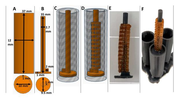
**Figure 2.** Views of CAD collagen injection molding chamber (**A**) and maturation plug (**B**) with dimensions displayed. CAD collagen injection molding chamber with maturation plug inserted (**C**) and with stent placement (**D**). Images of 3D printed actual crosslinked polyvinyl alcohol (XL-PVA) stents, over a maturation plug (**E**) and with the injection molding chambers (**F**).
