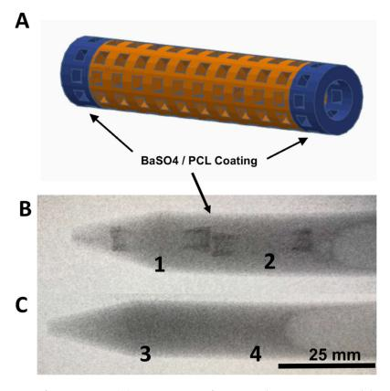
**Figure 3.** Images of CAD stent in (**A**), X-ray images of 3D printed XL-PVA stents with barium coated tips (**B**; 1 and 2), and X-ray image of control XL-PVA stents (**C**; 3 and 4). Black arrows point to regions of interest containing barium sulfate (scale bar = 25 mm).
