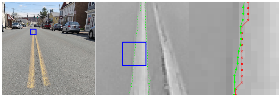
Figure 12. Image of a street in Watervliet, NY, where we seek to localize the edges of the painted yellow lane markings. The red \times symbols denote pixel-level edge estimates and green dots denote the refined subpixel localization estimates. Original image collected by the authors with a personal camera.
