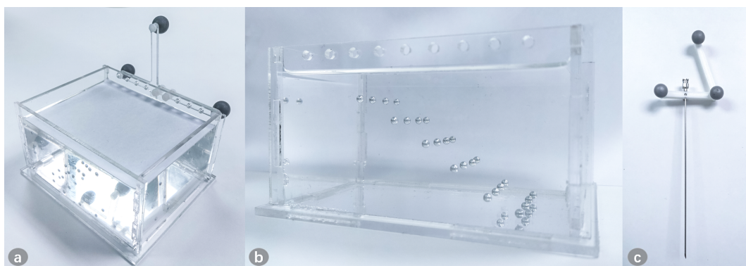
Figure 11. The model for puncture. (a) The model is fixed with the marker, and is covered to ensure that the surgeon cannot see the internal lesion information from above; (b) The lesions are placed at different depths, and the side of the model is transparent to check whether the needle successfully reaches the lesion; (c) The puncture needle is fixed with the 3D-printed reference.
