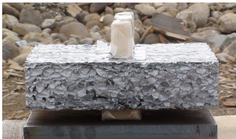
Figure 9. Block of Aluinvent continuous casted aluminum foam with an 85 mm thickness and 15 mm sized bubbles for a blast mitigation test with explosives shortly before detonation (courtesy of Norbert Babcsán, Aluinvent).
