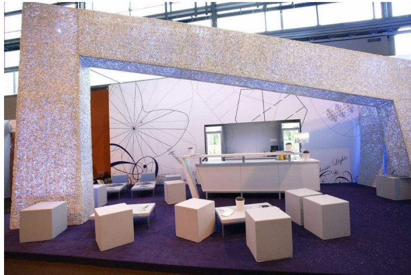
Figure 18. Booth for the convention center with an Alusion foam structure (courtesy of Alusion).
