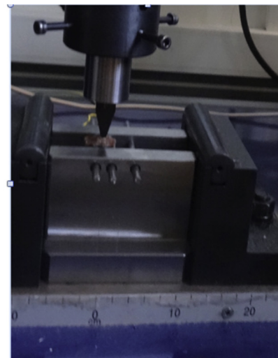
Fig. 1. Three-point bending test machine and setup.
