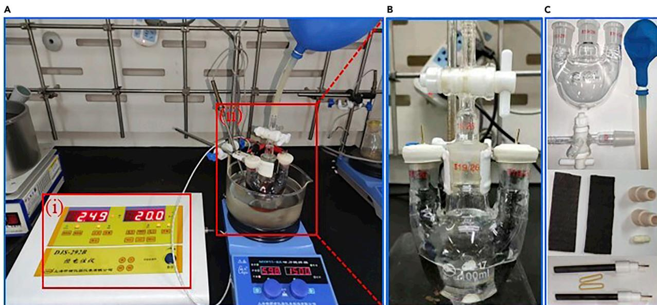
**Figure 1. Overview of the electrosynthesis system**
