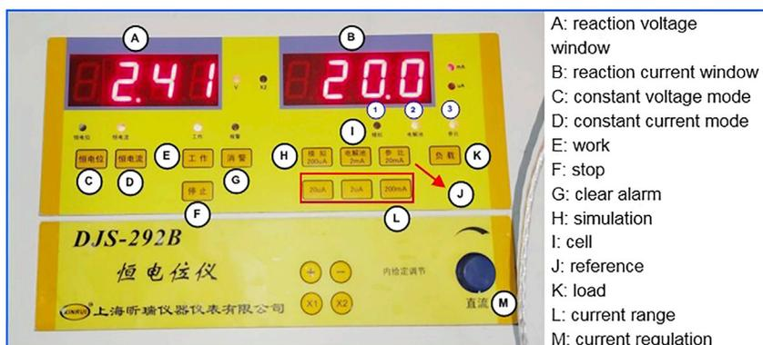
**Figure 2. DC power DJS-292B touch screen interface**
